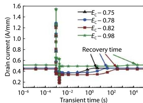
Fig. 6. (Color online) Current collapse and recovery curve, showing intentional doped Fe causes most of the current collapse and Ge doping caused current collapse takes approximately 2 h to attain steady state value.
