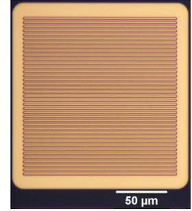
Fig. 3. Optical top view of a fabricated device with a  $W_{fin}$  of 2  $\mu\text{m}$  and a fin area ratio of 50%. The length of the fins is 150  $\mu\text{m}$ .
